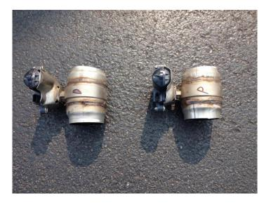
3) Remove the rear muffler assemblies from hangers. Squirting soapy water into the rubber hanger (Note: Soapy water does not hurt the rubber like WD40 could) will make removal easier. A large set of channel lock pliers to squeeze the hanger out of the rubber is recommended. Take care to not damage the exhaust tips during removal as they will need to be reused.
