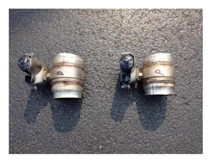
3) Remove the rear muffler assemblies from hangers. Squirting soapy water into the rubber hanger (Note: Soapy water does not hurt the rubber like WD40 could) will make removal easier. A large set of channel lock pliers to squeeze the hanger out of the rubber is recommended. Take care to not damage the exhaust tips during removal as they will need to be reused.
