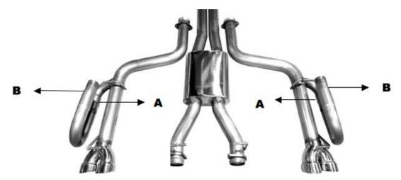
The J-pipes come to you with band clamps on them. The lower band clamps (A) need to be loosened and the J-pipe swiveled into the cavity where the stock muffler was. The J's are shipped resting on the tailpipe. This position is for shipping only. Once you install the system Clamp A must be loosened and the J-pipe turned away from the tailpipe into the muffler cavity. There is no correct position other than the J can't be touching anything and it must have clearance from the floor.
