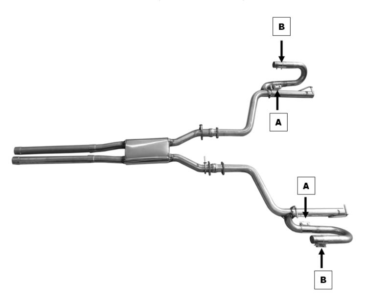
Note: The J-pipes come to you with band clamps on them. The lower band clamps (A) need to be loosened and the J-pipe swiveled into the cavity where the stock muffler was. The J's are shipped resting on the tailpipe. This position is for shipping only. Once you install the system Clamp A must be loosened and the J-pipe turned away from the tailpipe into the muffler cavity. There is no correct position other than the J can't be touching anything and it must have clearance from the floor.
