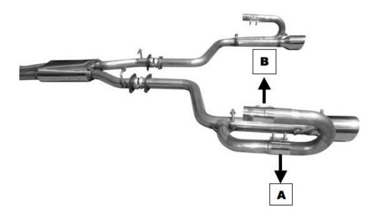
**Note:** The J-pipes come to you with band clamps on them. The lower band clamps (A) need to be loosened and the J-pipe swiveled into the cavity where the stock muffler was. The J's are shipped resting on the tailpipe. This position is for shipping only. Once you install the system Clamp A must be loosened and the J-pipe turned away from the tailpipe into the muffler cavity. There is no correct position other than the J can't be touching anything and it must have clearance from the floor.
