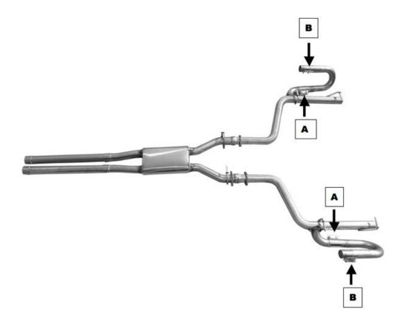
into the cavity where the stock muffler was. The J's are shipped resting on the tailpipe. This position is for shipping only. Once you install the system Clamp A must be loosened and the J-pipe turned away from the tailpipe into the muffler cavity. There is no correct position other than the J can't be touching anything and it must have clearance from the floor.
