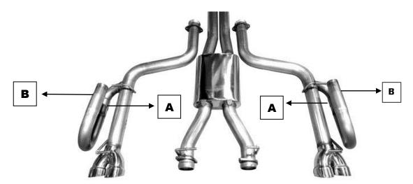
Note: The J-pipes come to you with band clamps on them. The lower band clamps (A) need to be loosened and the J-pipe swiveled into the cavity where the stock muffler was. The J's are shipped resting on the tailpipe. This position is for shipping only. Once you install the system Clamp A must
